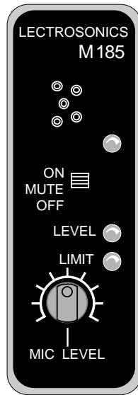
Figure 2 - M185 Front Panel
